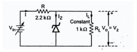
For  $V_{in(min)}$ ,  $I_Z = I_{Zmin} = 2.5 \text{ mA}$
