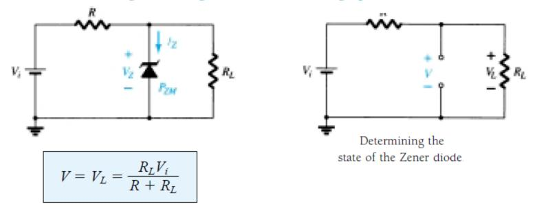
2. Substitute the appropriate equivalent circuit and solve for the desired unknowns.
