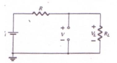
$$V_{i\min} = \frac{(R_L + R)V_Z}{R_L} = 23.67V$$
