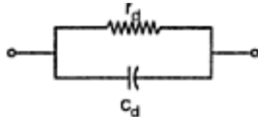
(c) AC equivalent circuit for forward-biased diode
