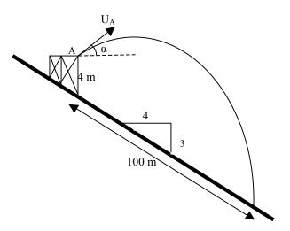
28. It is observed that a skier leaves the platform at A and then hits the ramp at B as shown in figure in 5 seconds. Calculate the initial speed  $U_A$  and the launch angle  $\alpha$ .
