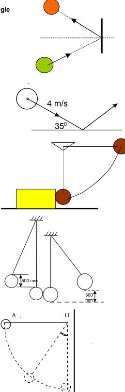
14. A ballistic pendulum consisting of a block of mass 30kg suspended from two wires each of length 1.8m is used to measure the muzzle velocity of the gun. If the pendulum swings through a horizontal distance s=25cm when a 40gm bullet is fired into it, determine the muzzle velocity v of the gun.
