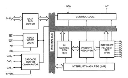
Internal block diagram of 8259A consists of 8 main blocks :
